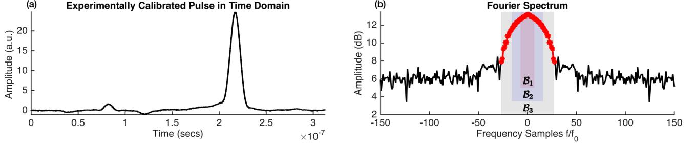
**Fig. 1:** (a) Time-domain samples of pulse  $\{\phi(nT)\}_{n=1}^{4464}$  calibrated using time-resolved sensor in [10]. Note that the pulse is smooth and asymmetric. (b) Fourier domain samples. Here  $\mathcal{B}_k = [-\Omega_k, \Omega_k]$ ,  $k = 1, 2, 3$  are possible bandwidths (for deconvolution) that can be used for super-resolving spikes.
