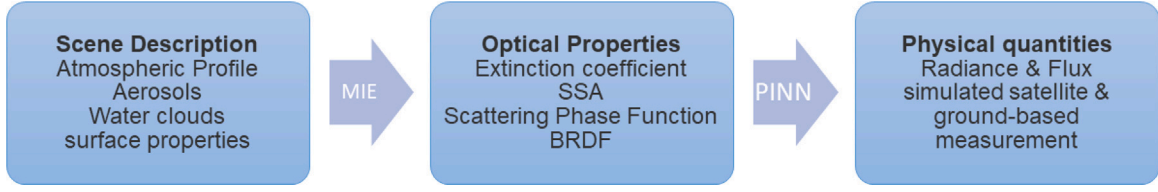
Fig. 2. Flow chart describing simulation process using RTPINN, the optical properties can either be generated by the standalone software or by the Libradtran code.
