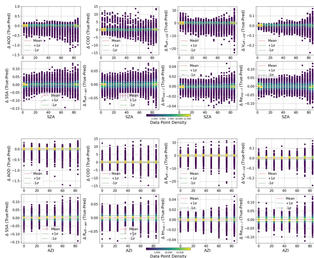
Figure 10. The difference between the true test and the predicted values versus SZA (upper panel) and AZI (lower panel). Test results are based on training a ViT network using two input vectors (I,Q) and normal distributions of all variables. Mean (dashed red line) represent the mean difference values with 1 standard deviation lines shown around the mean (dashed green lines). Colormap represents the number density of test points.
